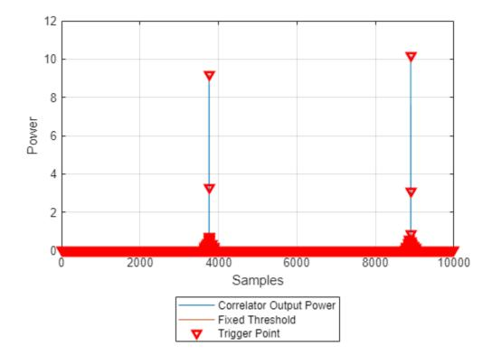
Choose a threshold value that is below any of the trigger point values. Plot the threshold information again and adjust the fixed threshold until the trigger points appear only on the correlator output peak.
