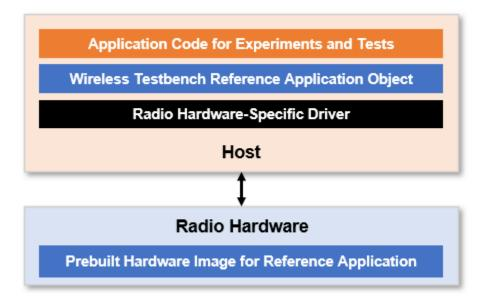
Using a Wireless Testbench reference application object, you can configure the prebuilt hardware image to transmit, capture, or detect wireless signals and write your application code for experimenting and testing.
