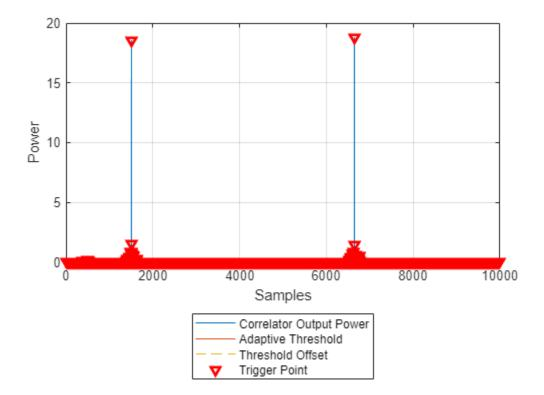
To remove all the trigger points from the bottom of the plot, set the adaptive threshold offset to a value that is above the noise floor. Adjust the adaptive threshold gain and plot the threshold information repeatedly until the correlator output is greater than the adaptive threshold.
